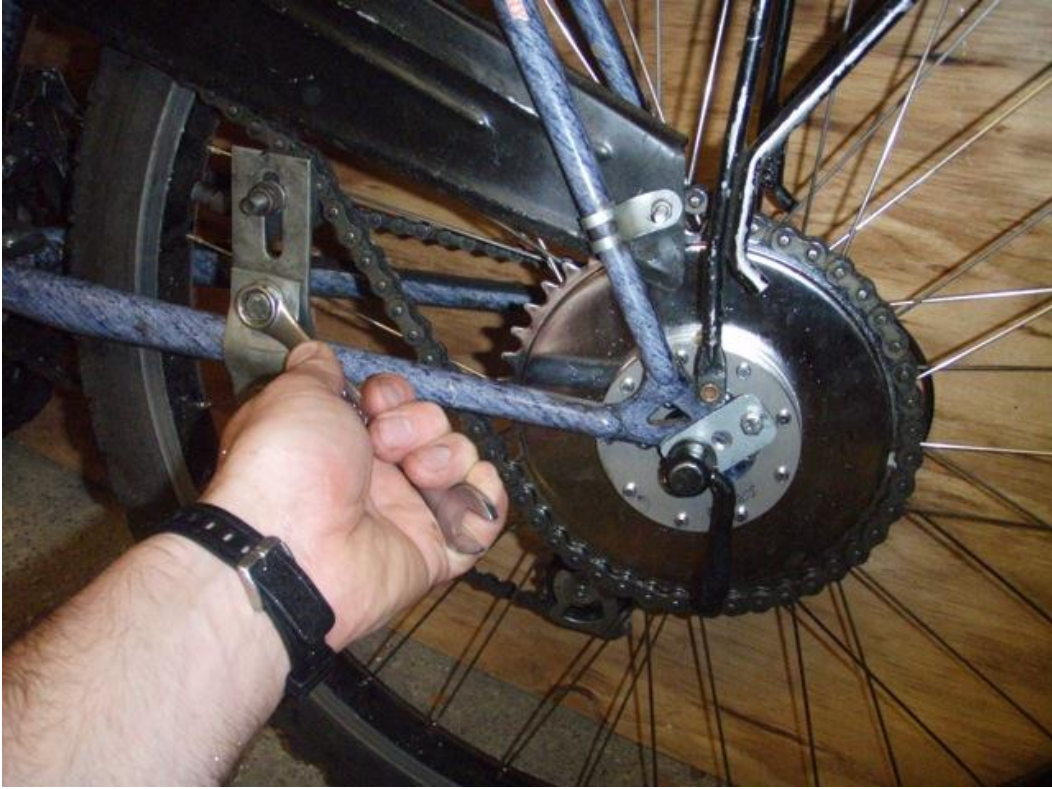
Step 4: Adjust the chain tensioner away from the wheel slightly to improve chain tracking.
