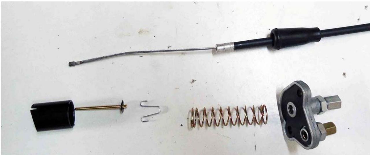
Firstly slide the needle into the hole in the center of the throttle slide as shown in Fig 4
